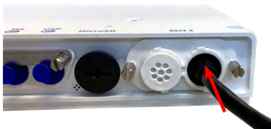
Fig. 24: Press the plug in firmly until the blue sealing ring clicks into place
