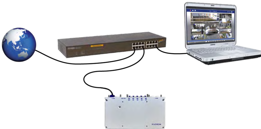
Fig. 23: Power supply using PoE switch according to PoE Plus (802.3at-2009)
